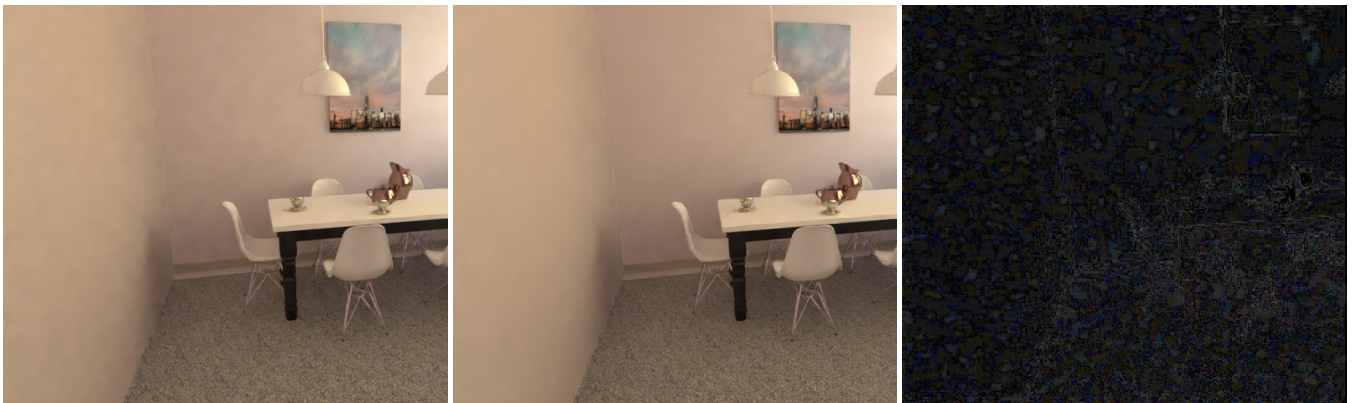
FIGURE 15: From left to right: without multiscale denoising , with multiscale denoising , relative absolute diff between the two . With multiscale compositing, most of the low-frequency noise on the walls (and everywhere else) goes away. The base single-frame denoiser is the same in both cases; the only difference is that in the multiscale setting we operate at multiple scales and blend the results.
