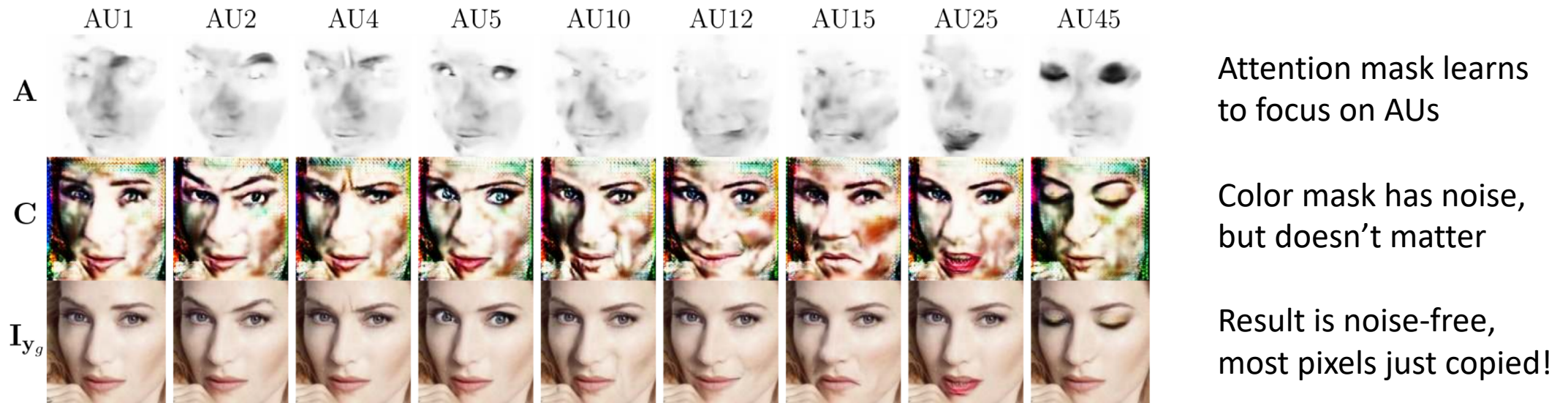
Fig. 5. Attention Model. Details of the intermediate attention mask A (first row) and the color mask C (second row). The bottom row images are the synthesized expressions. Darker regions of the attention mask A show those areas of the image more relevant for each specific AU. Brighter areas are retained from the original image.
