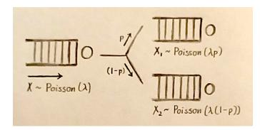
Poisson splitting. Each box-like entity represents a queue; each circle represents a server. Packets come in at the rate given by X. At the junction, packets go up the top path with probability p and down the bottom path with probability (1-p). We can see that the weights for the individual distributions are split accordingly.
